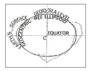
2.10 Biaxial ellipsoid as a normal body of the Earth
